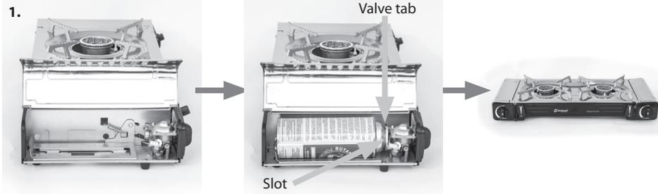
Open the gas cartridge compartment to fit the gas cartridge. Visually inspect the gas cartridge before you fit it to your appliance. Ensure that the nozzle is undamaged and in good condition. If the gas cartridge is damaged in any way do not attempt to fit it to your appliance. The control knob must be in the OFF position before connecting to the gas cartridge. Insert the gas cartridge into the holder so that the valve tab is aligned with the slot in the cartridge rim. Close compartment.
