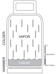
The Gas Level Indicator is a highly sensitive thermometer that measures the temperature change on the outside of the tank caused by the evaporation. This difference in temperature causes one or more columns on the Gas Level Indicator to change color right where the tank changes temperature. The vertical indication is the most important. The level is indicated where the most bar changes color. The horizontal indication also measures the environment temperature.
